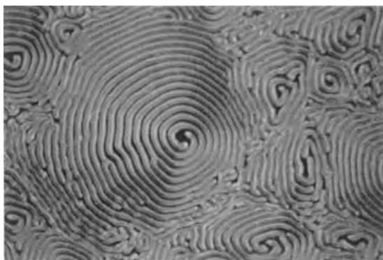
Fig. 3.8: Dislocations and other defects can be seen in the patterns formed by liquid crystals. Here, each ‘cell’ corresponds to a region of the liquid in which the rod-like molecules are aligned with one another in different directions. These differences can be revealed by illuminating the material with polarized light. Each sinuous domain here is just a few thousandths of a millimetre wide. (Photo: Michel Mitov, CEMES, Toulouse.)
